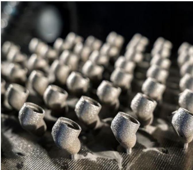
Figure 2: Automated series process in 3D printing via selective laser melting for the production of IE 600 housings
